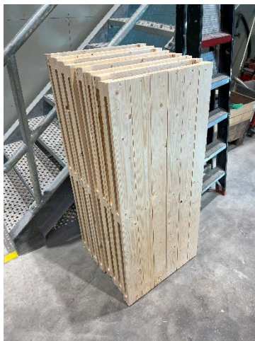
FIGURE 23: LINE BURNER TEST PANELS AS LAYERED WOODEN CONSTRUCTIONS
