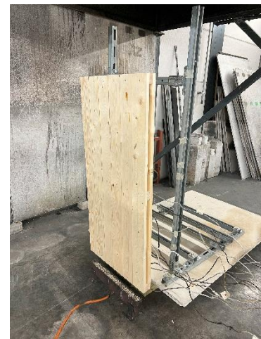
FIGURE 25: UNCOATED TEST PANEL CONNECTED TO THE TEST SETUP
