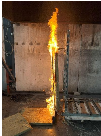
FIGURE 34: SIDE VIEW OF CHIMNEY EFFECT DURING LINE BURNER TEST
