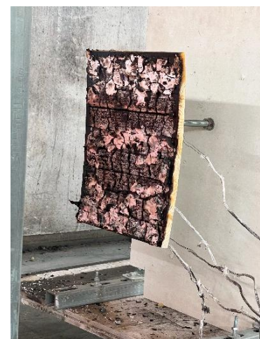
FIGURE 30: MYCELIUM AFTER THE TEST AND NO IGNITION
