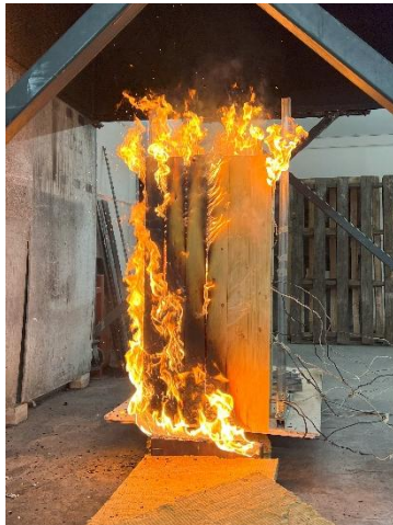
FIGURE 33: EARLY-STAGE DEGRADATION OF UNCOATED PANEL
