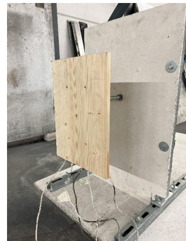
FIGURE 18: UNCOATED SPRUCE WOOD PANEL CONNECTED TO THE TEST SETUP
