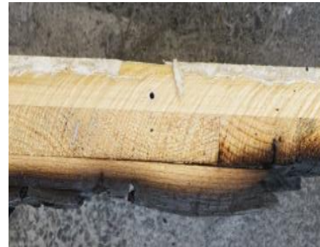
Adhesive that loses integrity upon heating
